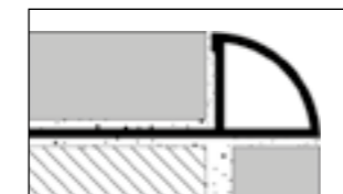
Wall tile corner
